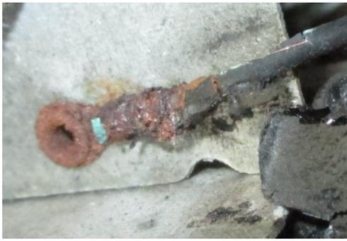
The remarkably rusted appearance of the terminals on the element caused suspicion that the hair-drier had spent time in a skip, or at least somewhere very damp.
